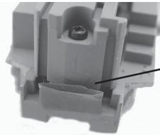
Use tape to completely wrap both front and rear ditch light board holders to prevent LEDs from touching the chassis
